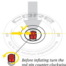
3. Check whether the valve is free from particles or obstructions.
